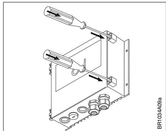
**The cover can be removed from the enclosure**
