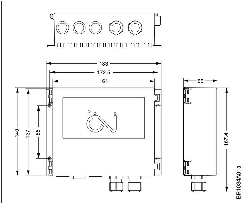
11.2 Stepper motor – dimensioned drawing
