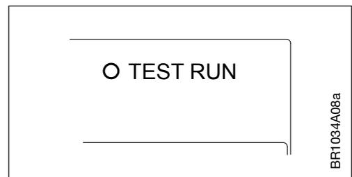
1. Pulley Calibration Test: Short press < 1sec.: The drive will enter test mode and stay in test mode until the button is pressed again. The motor will start rotating in a sequence from 0–100 rpm according to the selected ramp-up time and remain at 100 rpm for a minute, then stop and restart until a rotor guard error is shown.
